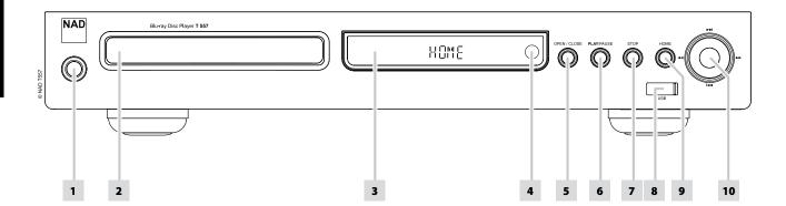
1 STANDBY: Press this button to switch ON the T 557. The display window will illuminate. If there is disc loaded, the display window will show the playback time status of the disc. If there is no disc loaded, the VFD will briefly show "NO DISC" and thereafter show the default display "HOME".
